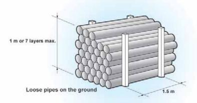
Racks for long term storage are recommended and should preferably provide continuous support, but if this is not possible then supports of at least 75mm bearing widths at 1m centres (max) should be placed beneath the pipes. Side restraints should be placed at centres not exceeding 1.5m and stacks should not exceed 1m in height.
