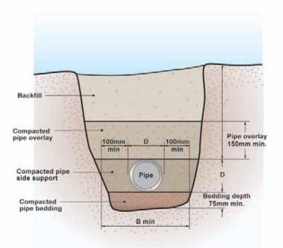
AS/NZS 2032 suggests the following materials as suitable for bedding and overlay in the trench:
