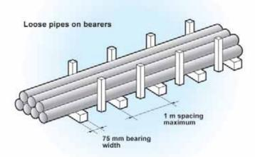
When unloading alongside dug trenches, it is recommended that pipes be placed on the opposite side of the trench from excavated material.
