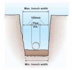
Trenches when excavated are either 'stable' or 'unstable'. The category into which a trench fits is affected by the soil conditions, width, depth and method of excavation. To ensure that maximum support is given to the buried pipe by the undisturbed ground the resultant stable or unstable trench should be treated in the following way:
