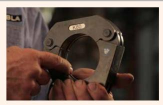
6. Select the appropriate sized KemPress® collar, check it is clean and that the surface of the pressing area is smooth.
