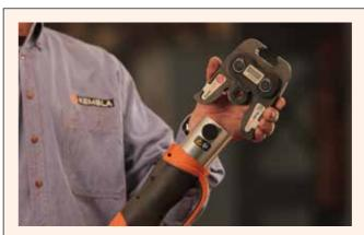
8. Select the ZB203 Adaptor Jaw, insert onto the KPL/ KPL2 pressing tool and arrest the locking bolts of the tool.
