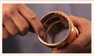
**3.** Ensure you have the correct sized fitting, check the fitting is clean and the stainless steel grip ring and O-ring are free from debris and correctly seated in the fitting.
