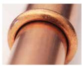
Unpressed fitting - small gap between fitting and tube.
