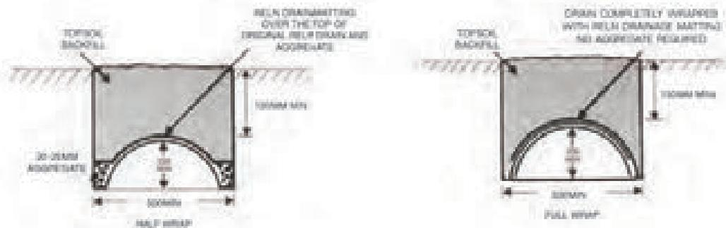
1. Dig trenches to suit your Rein Drain installation. Trenches should be level along the contour of the land to provide a uniform loading of liquid to the soil. Trenches must be at least 150 mm deeper than the top of the Rein Drain and deep enough to allow the required fall for pipework. On sloping land the first trench of Rein Drain should be fully utilised before overflowing into the next Rein Drain trench.
